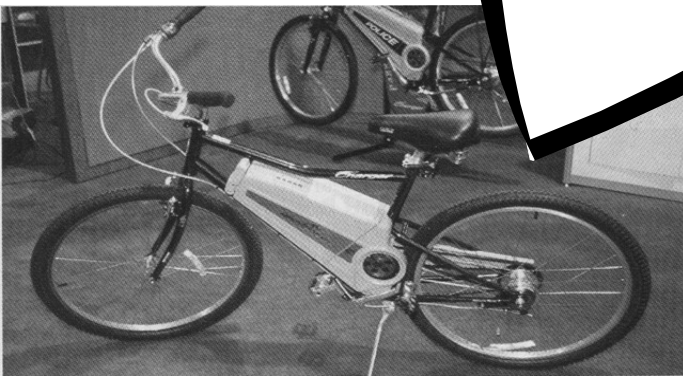
▲ The Charger electric bicycle is a joint effort between GT Bicycles and Aerovironment. Unlike other electrics, Charger is a pedal-assist design and will not operate unless pedaled. The rider selects one of four levels of boost and the motor makes everything feel like a downhill ride. Range is up to 30 miles on a charge. ( www.charger.com )
